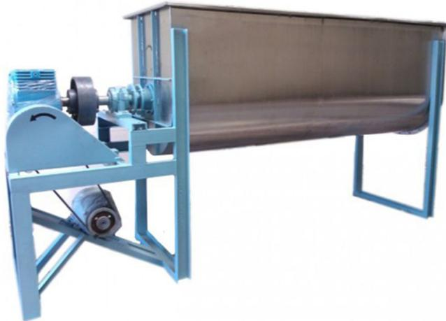
We offer a ribbon blender to our clients for their various industrial needs. The ribbon blender and their sides are manufactured by us from Stainless or Mild steel materials. It comprises of a stainless steel or mild steel centre shaft fitted with specially designed agitator blades for providing the contra flow action. These blenders are equipped with a couple of ribbons. The outer ribbon moves the ingredients into the blender whereas, the inner ribbon constantly circulate the material.
